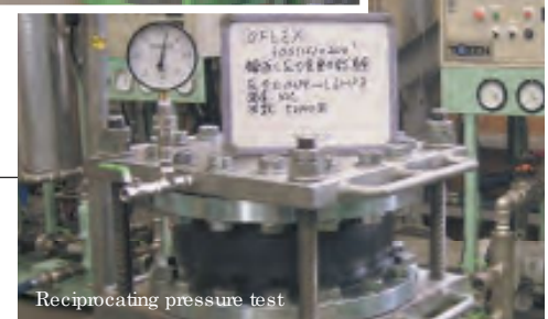
Reciprocating pressure test
